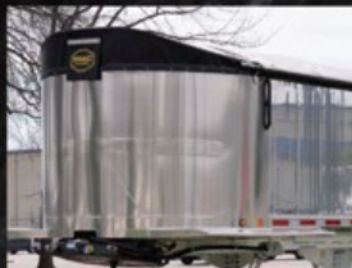
Optional tapered 84" to 90" front to back wedge body design
