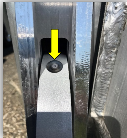
Figure 8-5 Top Overslung Rear Gate Pivot Pin and Latch Grease Fittings
