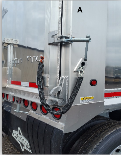
Figure 5-2 Open Winder on Tailgate
