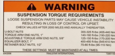
#295115000 Spring Suspension Torque Chart Rear of Frame Dr Side If Required
