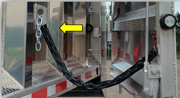
Figure 5-6 Anchor Door in Open Position
