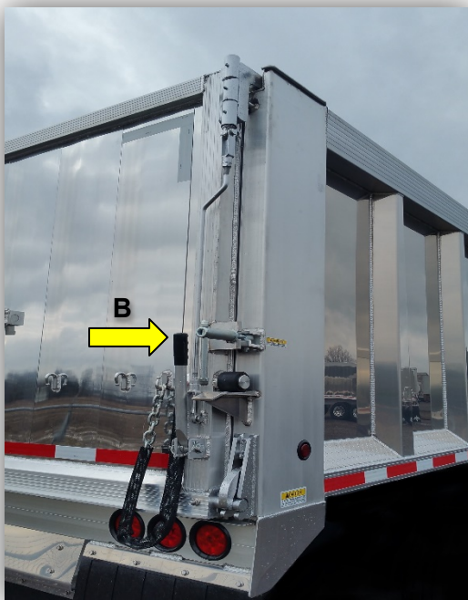
Figure 5-5 Pull Down on Ground Control Handle
