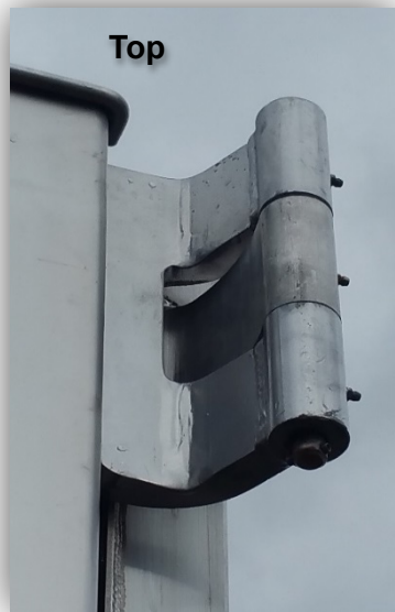
Figure 5-3 Side Swing Hinges Properly Engaged
