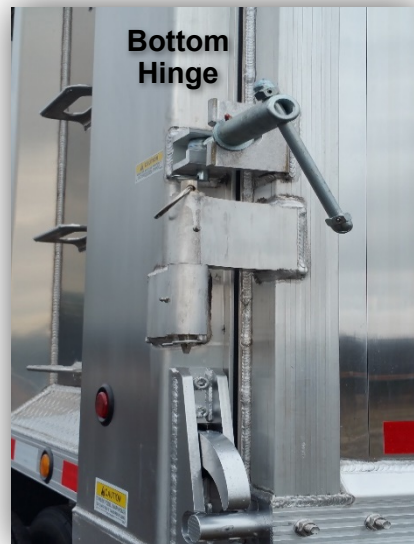
Figure 5-3 Side Swing Hinges Properly Engaged
