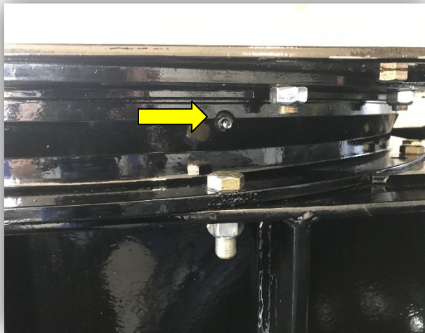
Figure 8-6 German Bearing and Frameless 5th Wheel Plate Grease
