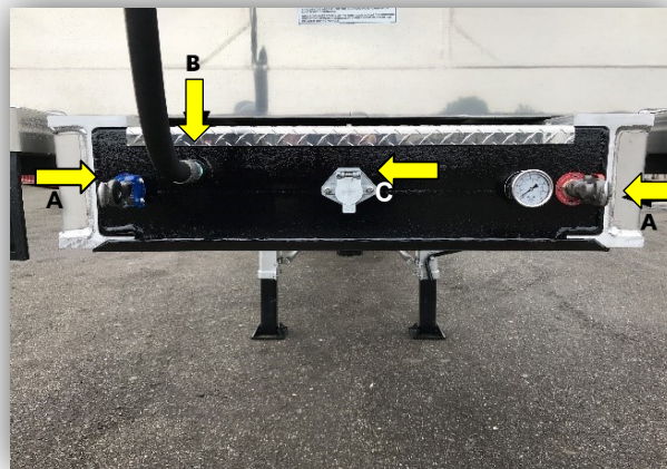
Figure 6-5 Disconnect Hoses and Electrical Connector
