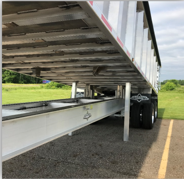
Figure 8-1 Block Up Dump Body
