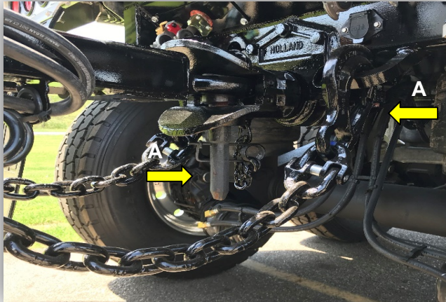
Figure 6-2 Disconnect Safety Chains, Hydraulic Hose
