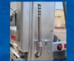
Manual Gate Ground Control
