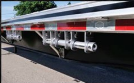
Load securement: J-track in floor, chain tie downs, or double LL winch track with galvanized winches
