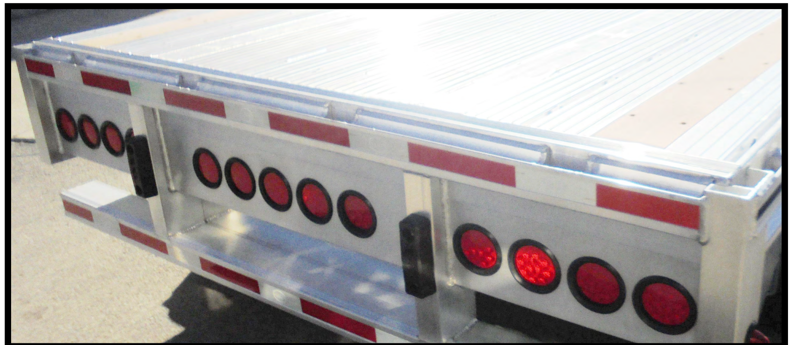
MAC Trailer Shown With Integrated Skid Seats In Rear Light Panel
